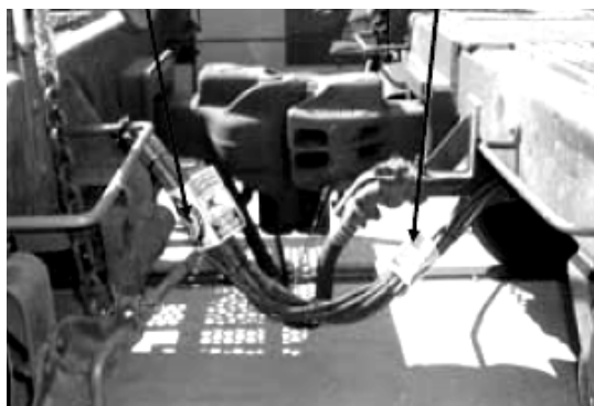
Electrical Cable Strung between Cars with affixed warning signs:
